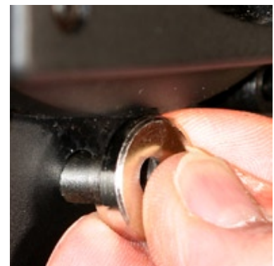
1) Grasp the Emergency Eject Knob
